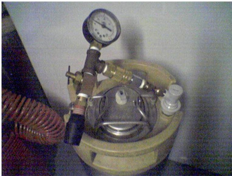
Illustration 4 Attached to a single fermenter for pressure testing or fermenting under pressure
