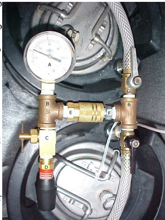
Illustration 1A device for secondary fermentation with controlled pressure relief to retain natural carbonation
