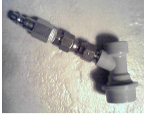
Illustration 3 Adapter for single keg fermenting or pressure testing
